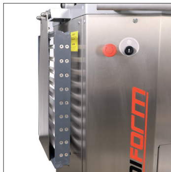
Left side grid storage
