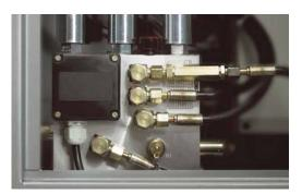
Silent long life hydraulic pressure system. Standard on Variomatic and an interesting option on other models: variable pressure regulation for any dough type.
