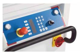
Programmable pressing and rounding times ensure better product consistency. Because the machine runs through its cycle automatically, a higher output is achieved.
