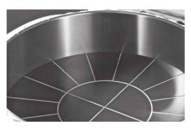
A Teflon<sup>®</sup> coated cast-iron dividing disc with stainless steel knife and ring around the dough tub require less flour and make the Robocut robust and hygienic.
