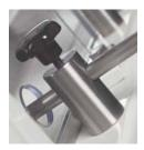
The side guides and the upper belt can be adjusted according to the length and height of the loaf.
