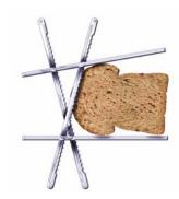
This innovative slicer is equipped with Daub's unique and proven cross-slice system. The loaf is cut at an angle with a longer stroke of the blades, which results in faster slicing (even fresh loaves) and a smooth and silent operation.
