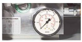
Standard on the Variomatic and an interesting option on other DR Robot models: variable pressure regulation for any dough type.
