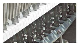
The patended saw tooth wave slice system handles all types of loaves. It uses unique robust Teflon<sup>®</sup> coated blades for extra long life span. Changing does not require a service technician.
