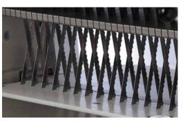
Thanks to the cross slice system, blades last up to three times longer than conventional systems.
