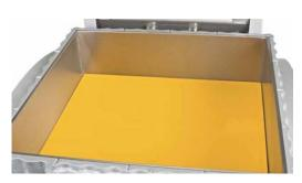
With the optional pressure plate, square versions of the Robocut can be used as dough or butter press.
