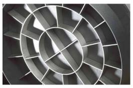
There's a choice of seven anodized coated aluminum dividing discs with stainless steel knives. The discs require minimal flour for dividing, are hygienic and can be cleaned in a dish-washer.
