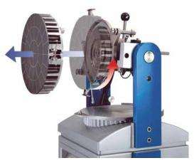
Interchangeable dividing disc (within 5 minutes) offers increased flexibility, a work range of 16-250 gr. and tilts forward for easy cleaning.
